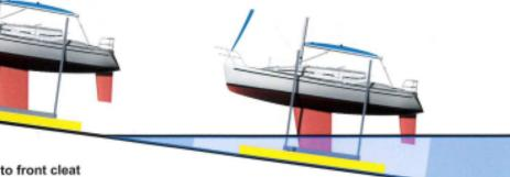
Attach rope to front cleat to prevent boat tipping back
