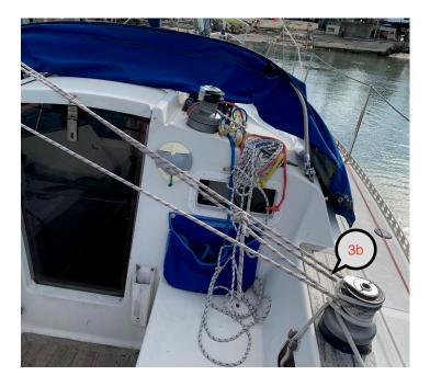
4. Rope tied to base of port winch, back to rear boat cleat, then to upright and back to top of winch. To stop yacht dropping backwards, when on the trolley.
